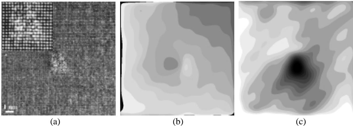
Fig. 4 : a) HRTEM image of a rod precipitate embedded in the Al matrix (AA6056-T6). As illustrated by the insert, the precipitate structure is quite ill defined and the matrix is highly deformed by the rod precipitate. b) Phase map obtained for a  $g_1$  direction c) Phase map obtained for the  $g_2$  direction. Fig. 4c clearly shows the asymmetry of the displacement field due to the rod.
