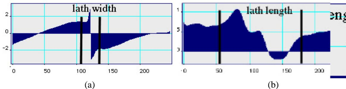
Fig 3: a) (resp. b) Profile of the displacement taken along a horizontal (resp. vertical) line cutting the lath. The phase range between  $(-\pi, \pi)$  which is linearly corresponding to a displacement 0.2 nm.
