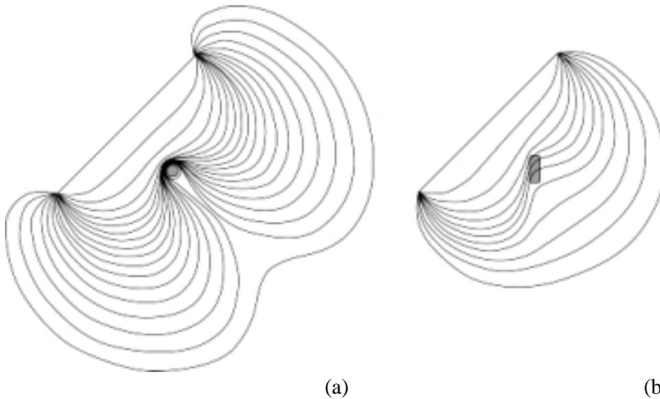
Fig. 5 : Comparison of the simulated movements of a  $1/2\langle 110 \rangle$  dislocation under a constant applied stress in the vicinity of a rod a) or of a lath b). The dislocation has been drawn for successive positions corresponding to a constant interval of time. Notice that the shearing of the lath starts at the small end of the lath, which corresponds to the lowest stressed area of the matrix near the surface of the lath.
