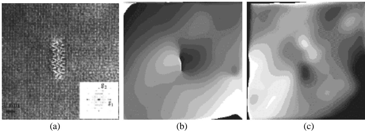
Fig. 2: a) HRTEM image of a lath precipitate embedded in the Al matrix (AA6056-T6) . b) Phase map obtained with the  $g_1$  selected vector c) Phase map obtained with the  $g_2$  selected vector
