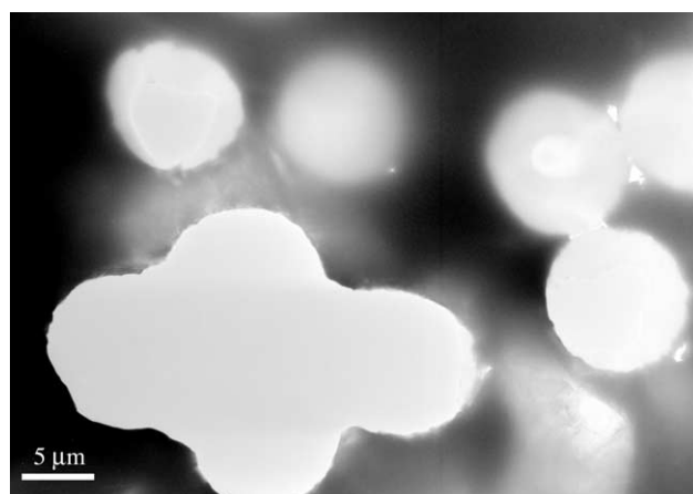
Fig. 6. Low magnified TEM micrograph of AlCu/C annealed composite. The carbon fibres appear undamaged.
