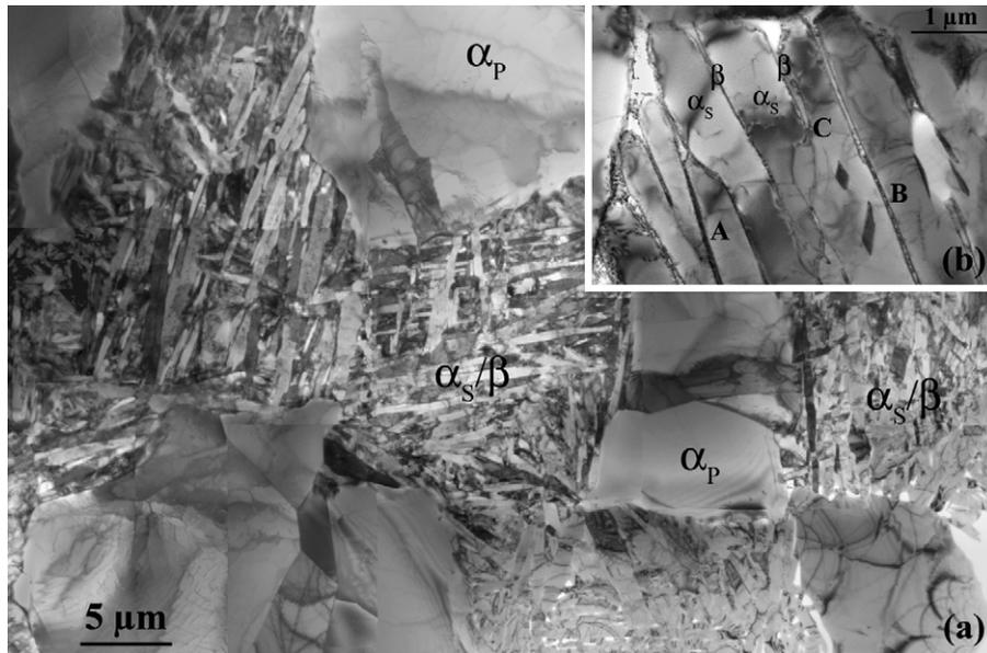
Fig. 1. TEM image of the general alloy microstructure (a) and detailed view of a lamellar colony (b).
