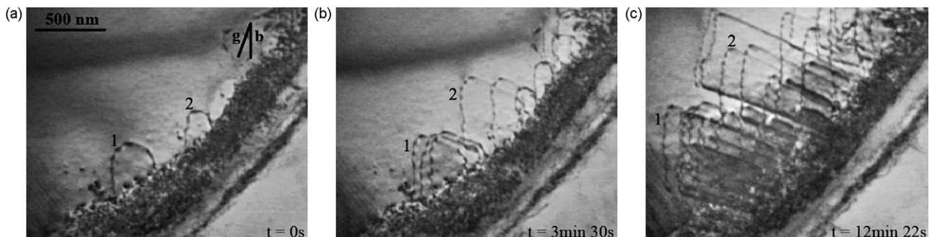
Fig. 2. In situ TEM observation of the dislocation emission from a  $\beta/\alpha_P$  interface.
