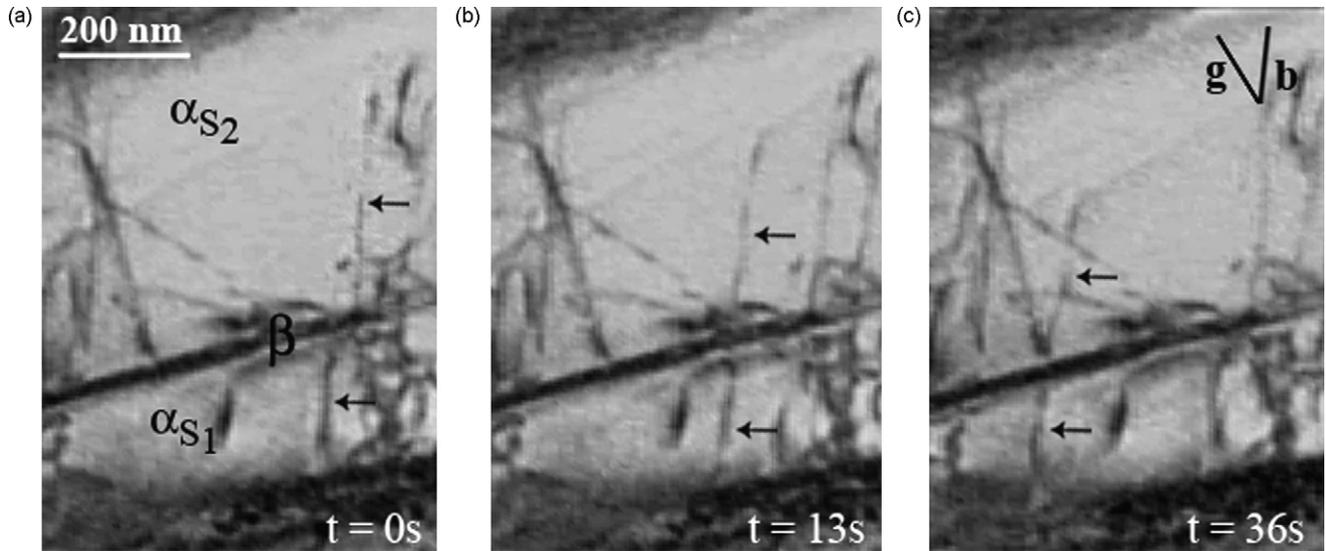
Fig. 3. In situ sequence showing simultaneous slip of dislocations in two  $\alpha_S$  laths and one  $\beta$  lath.
